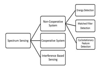
Fig. 2 Classification of Spectrum sensing technique.
