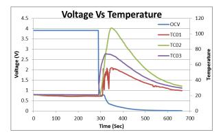
Fig. 8 Voltage and temperature relationship due to Flat plate deformation test
