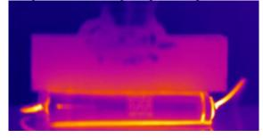
Fig. 5 Thermal hotspot of Flat plate deformation test
