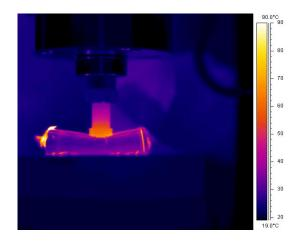
Fig. 3 Thermal hotspot of Rod indentation test
