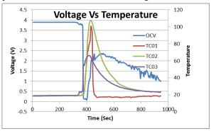
Fig. 6 Voltage and temperature relationship due to Rod indentation test
