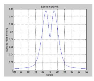
Fig 8: Electric Field Plot 132 KV Tower
