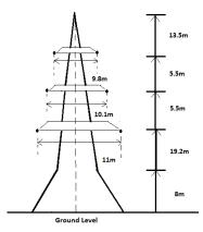
Fig 3: 220 KV Tower Configuration WAPDA
