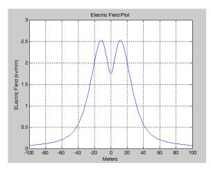
Fig 10: Electric Field Plot 500 KV Tower
