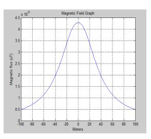
Fig 7: 500 KV Tower Magnetic Field (Merlin Conductor)
