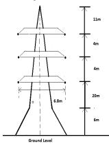
Fig 2: 132 KV Tower Configuration WAPDA
