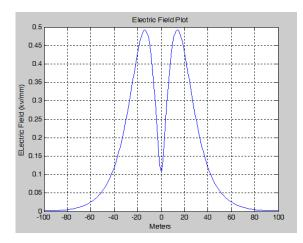
Fig 9: Electric Field Plot 220 KV Tower
