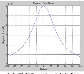
Fig 5: 132 KV Tower Magnetic Field (Rail Conductor)
