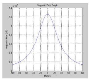
Fig 6: 220 KV Tower Magnetic Field (Curlew Conductor)
